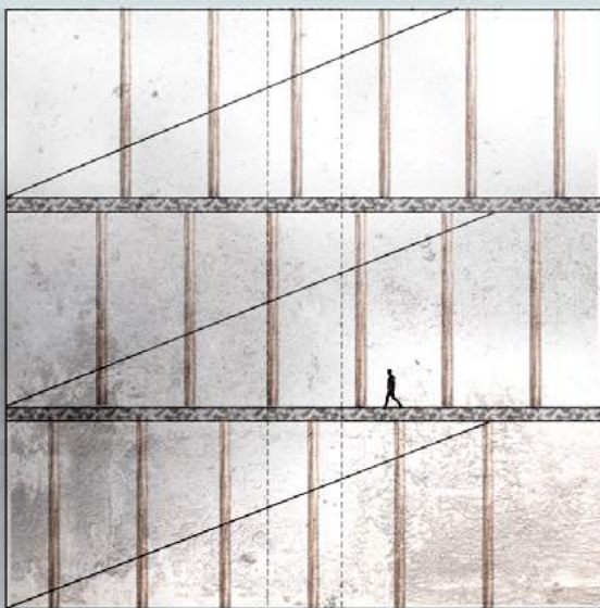
3.PARALEL RAMP SYSTEM (NOT OPTIMAL FOR CIRCULATION)
