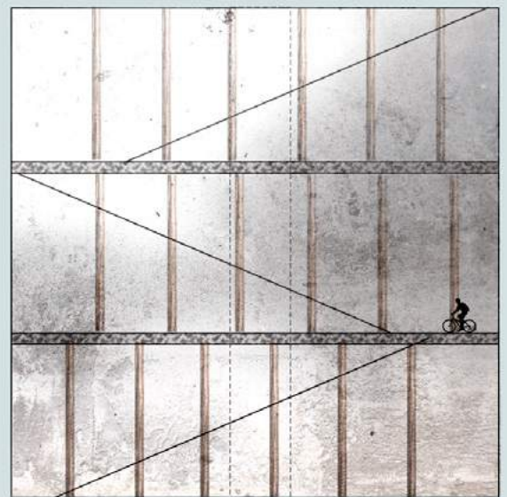
4.OPPOSING FINAL RAMP SYSTEM (OPTIMAL FOR CIRCULATION FLOW)
